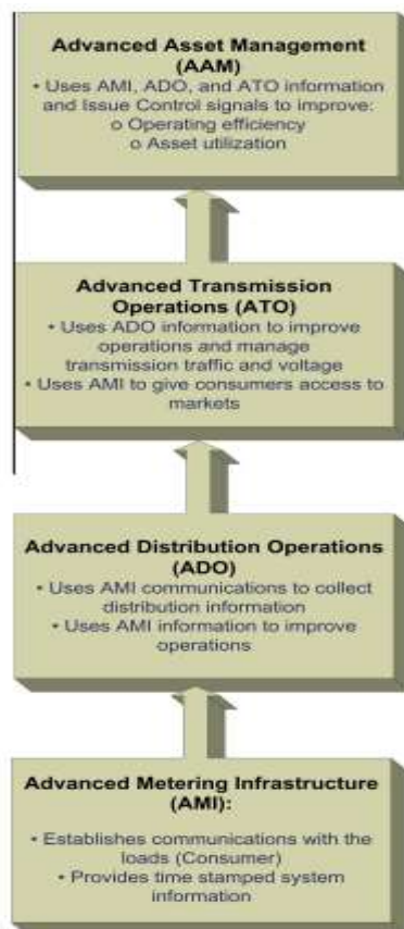
Fig. 1. An overview of Smart Grid sub-system sequence.
